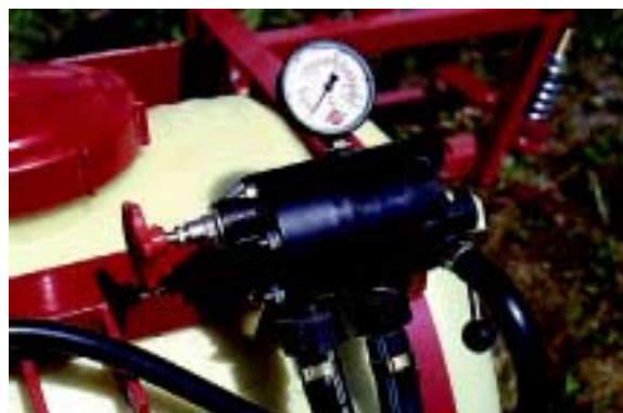
M-70 control unit showing pressure regulator, main on/off valve and pressure gauge.
